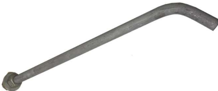
J-BOLT M25 x 570mm x 130mm THEARD H.D.G (WITH 2Hex Nut & 2Flat Washer)
